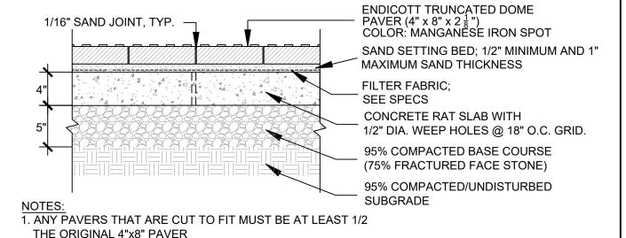
PEDESTRIAN TRUNCATED DOME BRICK PAVING - SECTION ENDICOTT TRUNCATED DOME 1/16" SAND JOINT, TYP. -PAVER (4" x 8" x 2 ½") COLOR: MANGANESE IRON SPOT SAND SETTING BED; 1/2" MINIMUM AND 1" MAXIMUM SAND THICKNESS  $\triangleleft$ 114 FILTER FABRIC; 8" 11 SEE SPECS  $\Pi$ CONCRETE RAT SLAB WITH 1/2" DIA. WEEP HOLES @ 18" O.C. GRID. 8" 95% COMPACTED BASE COURSE (75% FRACTURED FACE STONE) 95% COMPACTED/UNDISTURBED SUBGRADE NOTES:
