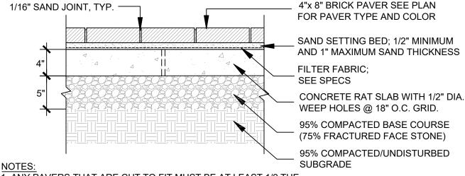
1. ANY PAVERS THAT ARE CUT TO FIT MUST BE AT LEAST 1/2 THE ORIGINAL 4"x8" PAVER.
