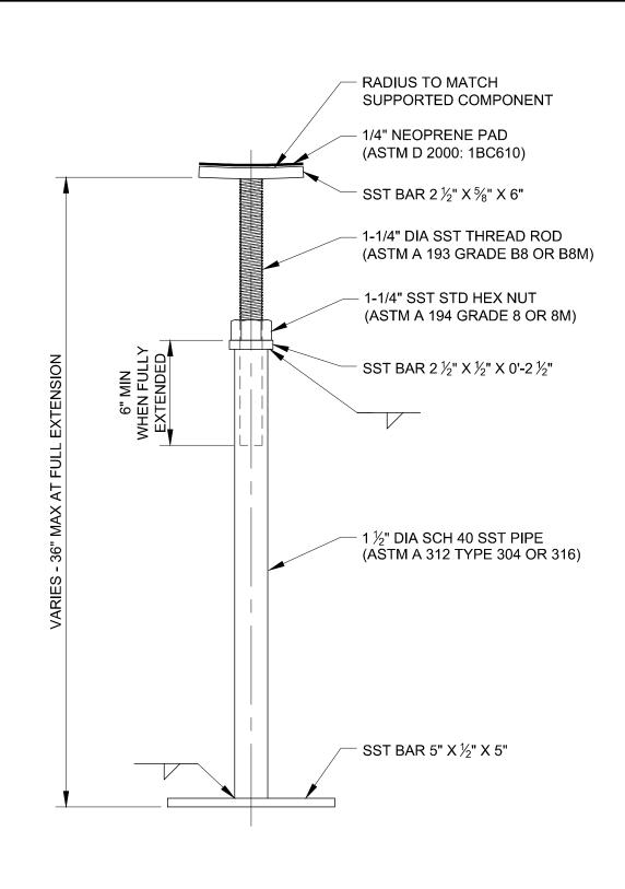
1. BAR MATERIAL TO BE ASTM A 240 TYPE 304 OR 316 (Fy= 30 KSI MIN.)
