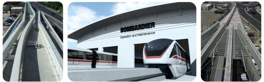
High speed beam replacement turn out switch
