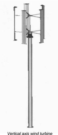
The overall diameter of the system is approximately 19.7 feet in diameter. Also proposed with this system (separate structure) is a sun tracking solar panel. The system's proposed location near the Silverlode Lift was analyzed over a multi-year period using anemometers and determined to be the best possible location.
