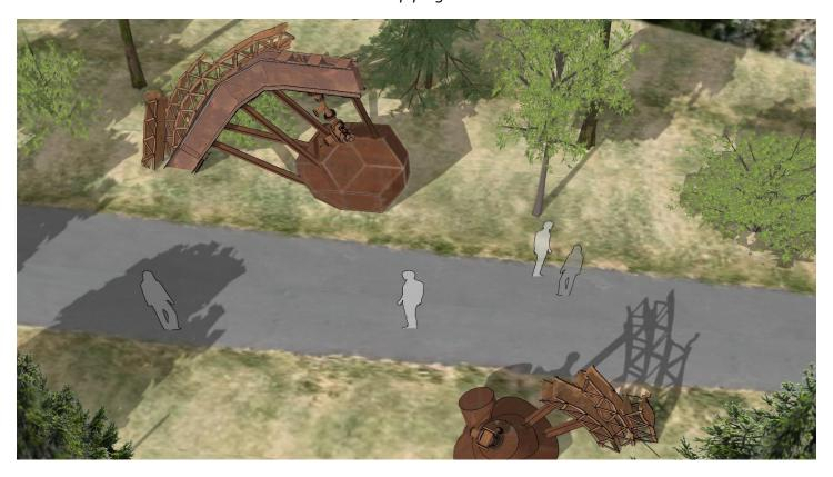
Figure 2: Aerial view. Steel hollow-forms serve as pour-forms for reinforced concrete to support the structure.
