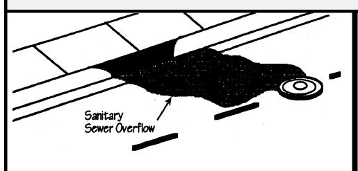
Implement control procedures for identifying, repairing, and remediating sewer blockages, infiltration, inflow, and wet weather overflows from sanitary sewers into the storm drain conveyance system. Procedures include field screening, follow-up testing, and complaint investigation.
