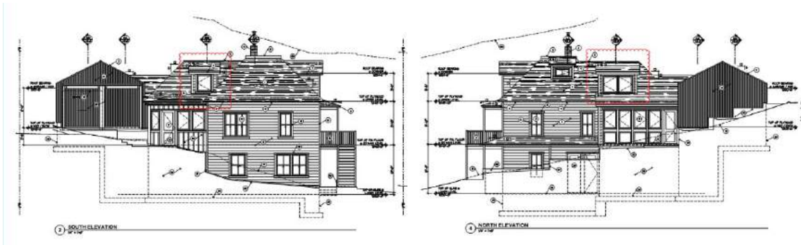
Location of new dormers on the reconstructed roof.
