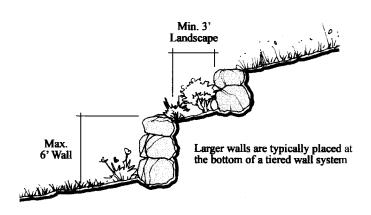
Tiered Retaining Wall Section
