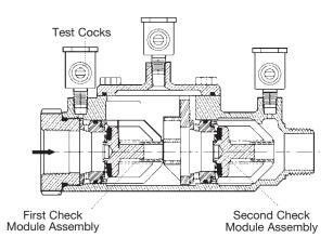
The LF007 Series features a modular design concept which facilitates complete maintenance and assembly by retaining the spring load.
