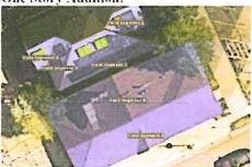
Relocation of the panels to the North/East roof of you building is not a good option. Relocation of your panels would result in a 65% production loss. The cost to relocate the panels would not be offset by the panels production.
