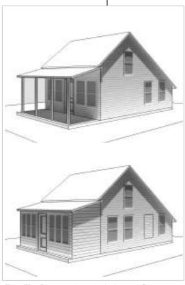
Top: The front porch and window configuration are original. Bottom: Window openings have been altered and the front porch enclosed. These treatments are incompatible and should be avoided.
