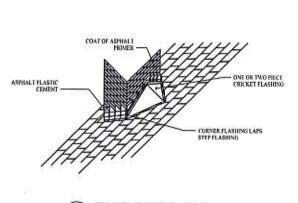
9 VENT FLASHING DETAIL
