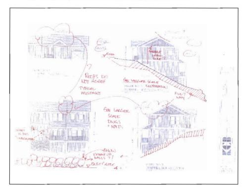
A void space 12' to 15' high below the garage on the downhill side, suggests the design is not well suited to the steep topography of the site. Earlier Site layouts concentrated the structures on "the flatter part of the site". Claims that this is now a more "clustered" development are absurd.
