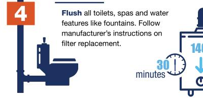
Increase the temperature on the hot water heater to at least 140 degrees for 30 minutes. Turn on the hot water tap closest
