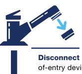
**Disconnect** any pointof-entry device filters and household filters and softeners and remove aerators. After flushing inspect and maintain before putting back in service.
