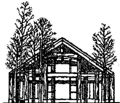
Fig 2-8: Large viewing windows shall be recessed under overhangs.
