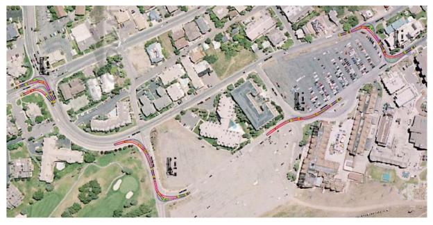
Overall view of the intersections evaluated for truck turning templates
