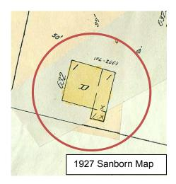
The applicants' research indicates that staff erred in the analysis presented to the HPB in November 2013 as staff found that the addition expanding the house from a rectangle to a square floor plan was added across the rear (south) elevation of the structure. The applicant suggests that the addition was actually added across the front (north) elevation of the structure.
